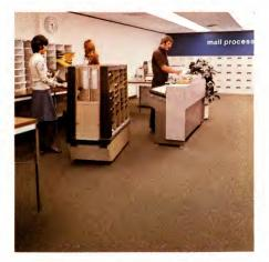
Mailmobile's time — and labor-savings begin right at its point of origin, the mailroom. Mail can be sorted directly into the delivery compartments, eliminating the need for double-sorting. Notice how the design complements other mail equipment in size, tray accessibility, and level of work surfaces.
